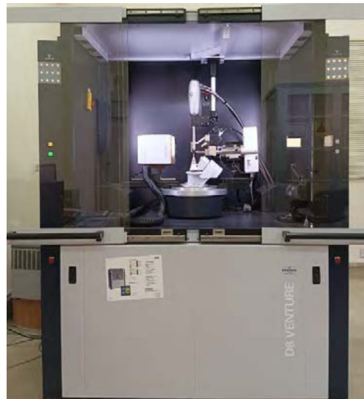
Bruker SMART APEX D8 Venture having Cu as source with CMOS 100 photon detector (Single Crystal XRD)
