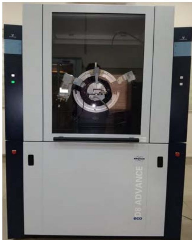
Bruker D8 ADVANCE Fitted with Cu as source with LYNXEYE-2 detector (Powder XRD)
