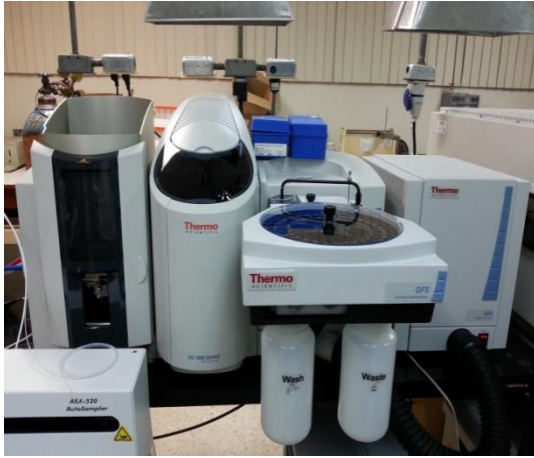
Thermo Scientific iCE 3500 AA Spectrometer with integrated graphite furnace
