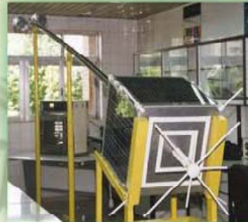
Fixed cross yagi antenna
