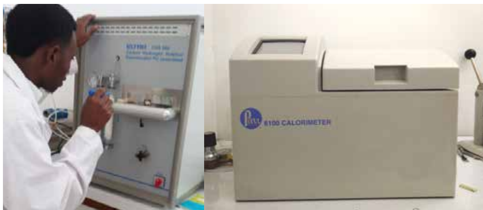
Figure-1: Coal Laboratory Equipment: CHS 580 for ultimate analysis (left) and bomb calorimeter for gross calorific value determination (right)
