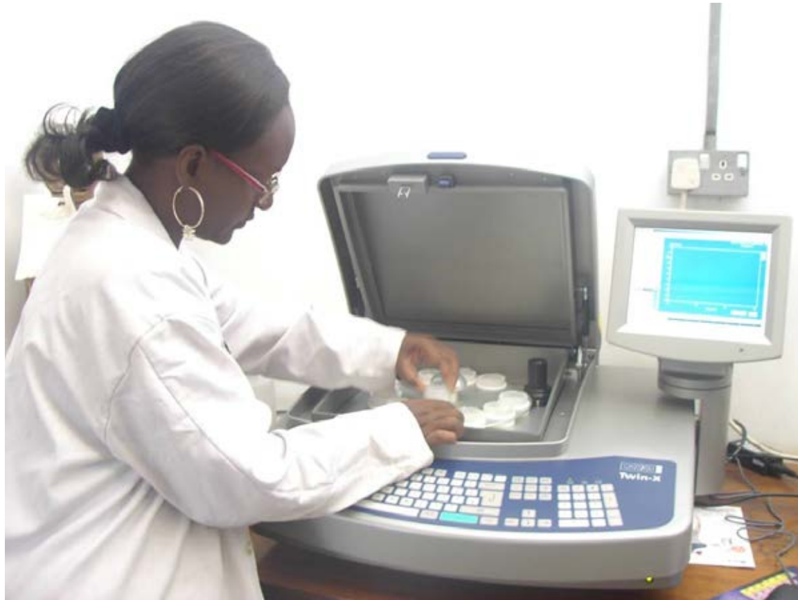
XRF machine for quantifying inorganic materials content
