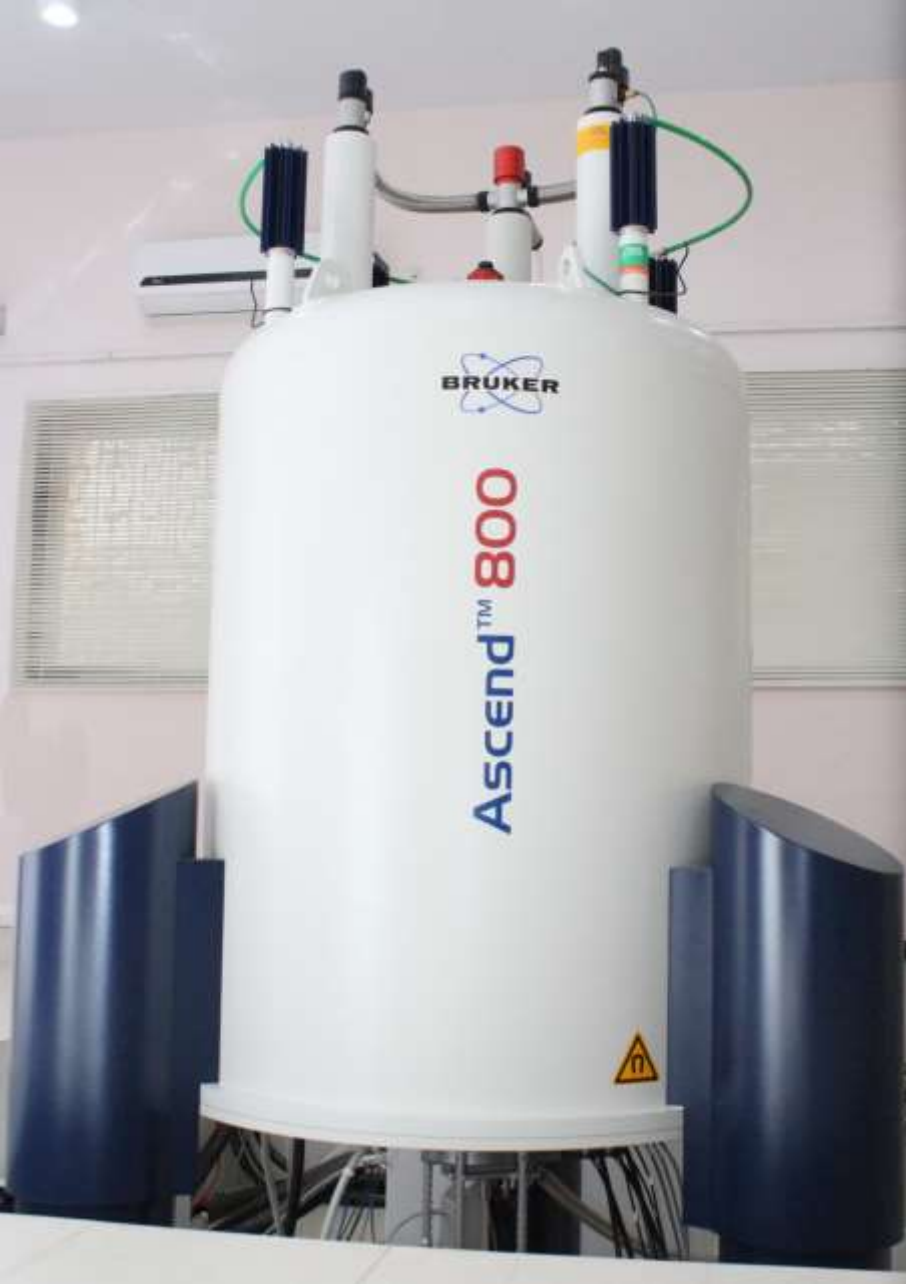
800 MHz Nuclear Magnetic Resonance (NMR) Spectrometer
