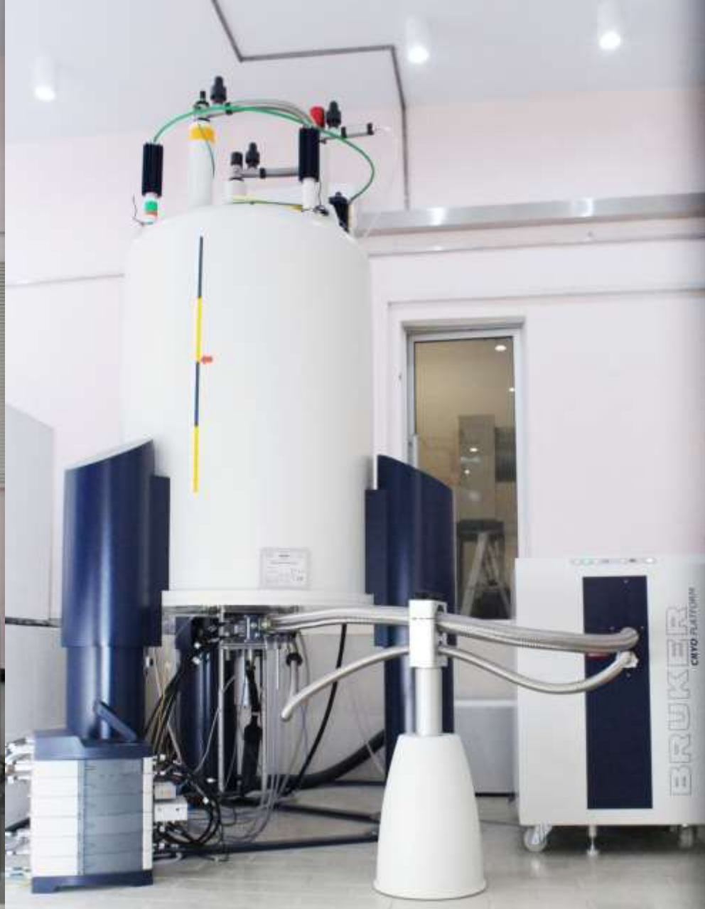
800 MHz Nuclear Magnetic Resonance (NMR) Spectrometer
