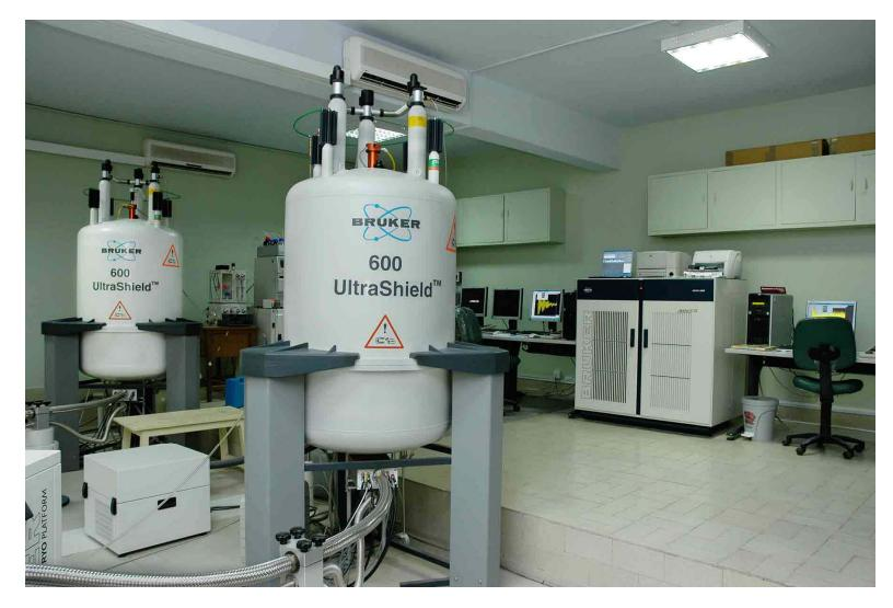
NUCLEAR MAGNETIC RESONANCE SPECTROMETERS
