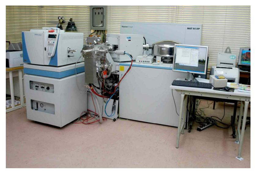
MASS SPECTROMETER (ELECTROSPRAY IONIZATION)
