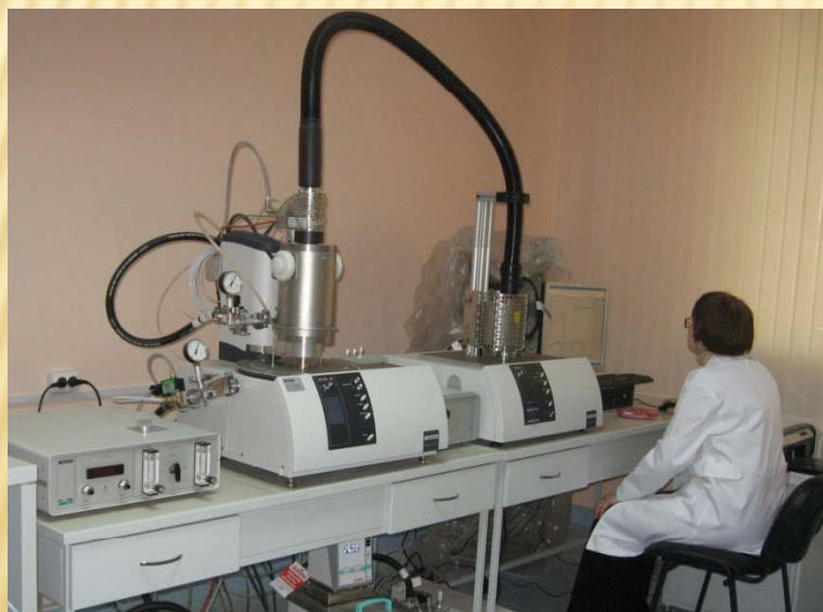
Synchronous thermal analyzer TG-DTA/DSK with quadrupole mass spectrometer : STA 449 F3 Jupiter® NETZSCH (Germany)
