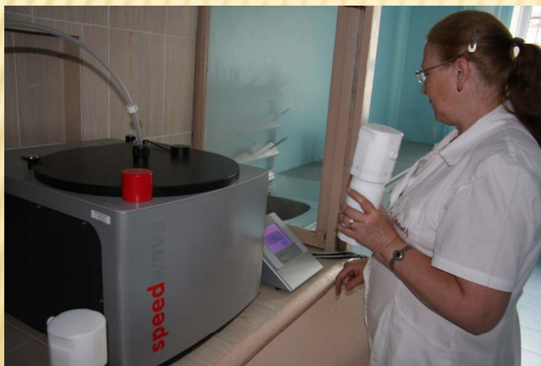
System of microwave decomposition with vertical feeding and temperature and pressure control function speedwave four BERGHOF(Germany)
