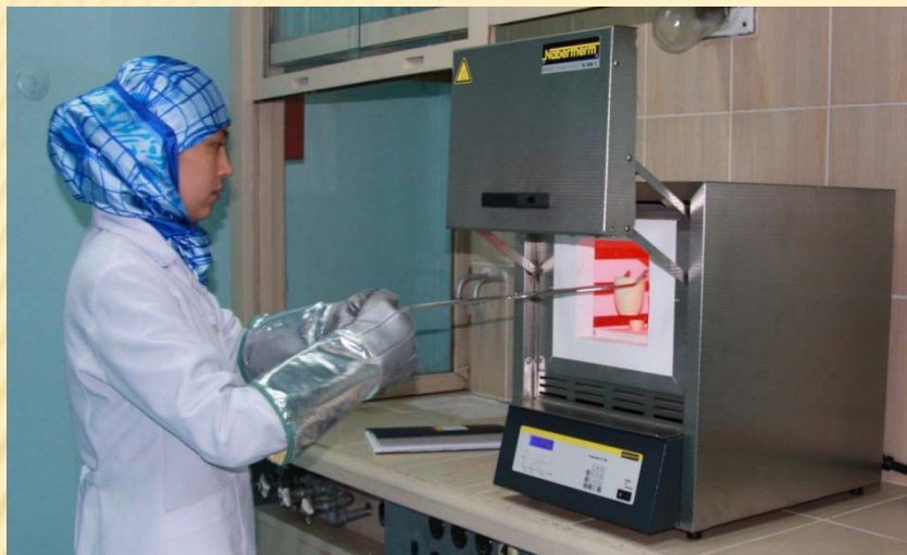
High-temperature chamber furnace 1600 °C HTC 08/16 (Nabertherm GmbH, Germany)
