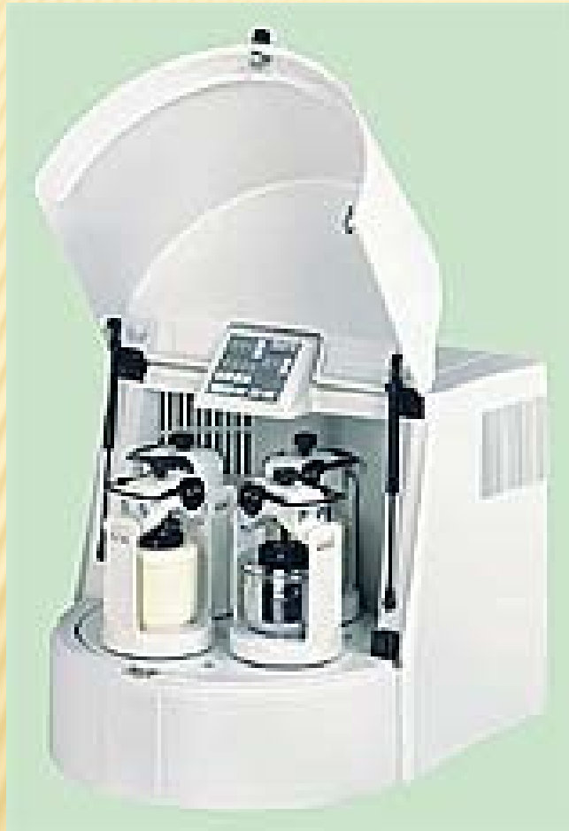
Planetary mono-mill Pulverizette 6 Fritsch GmbH (Germany)
