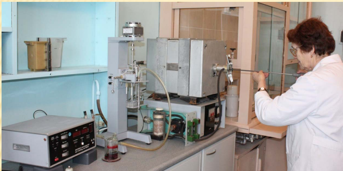
Express analyzer on carbon AN-7529M (Gomel instrument-making factory, Belarus)
