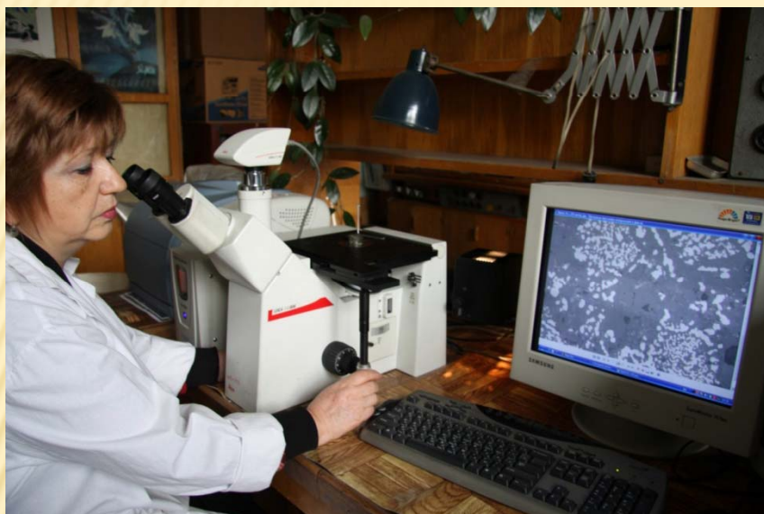
Metallographic workstation on basis of inverted microscope Leica DM IRM, «Vetclar», Germany
