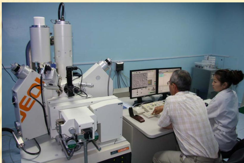
Electronic raster microscope with analyzer JEOL JXA-8230 (Japan)
