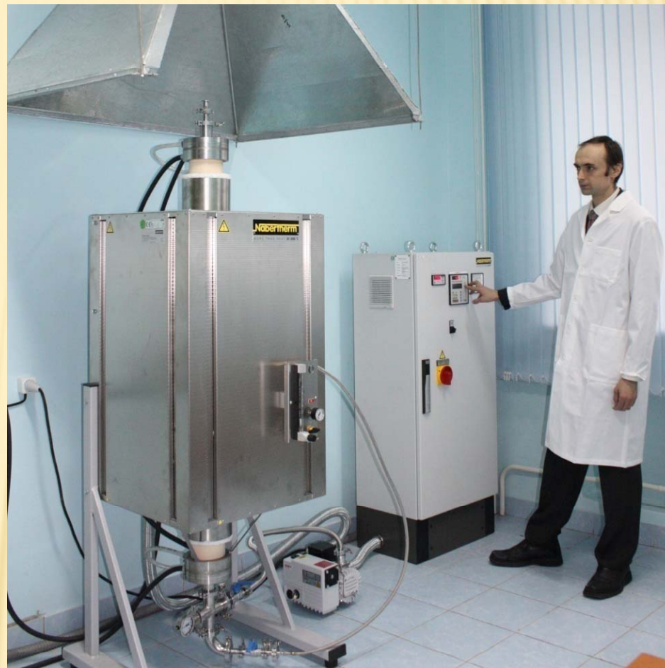
High-temperature tubular furnace 100/600 for vertical mode. RHTV 120-600/C 40 Nabertherm (Germany)
