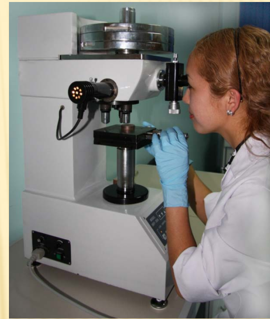
Multifunctional stationary hardness meter HBV-30A (Laizho huayin testing instrument co., LTD, China)
