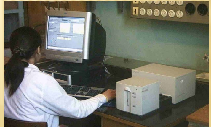
Spectrophotometer Agilent 8453 UV-Vis (Germany)
