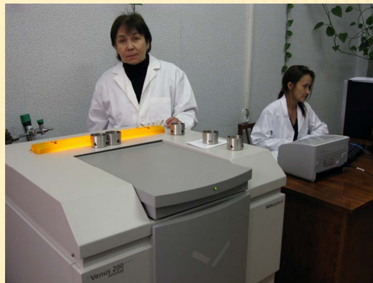
Roentgen fluorescent spectrometer with wave dispersion Venus 200 PANalytical B.V. (Holland)
