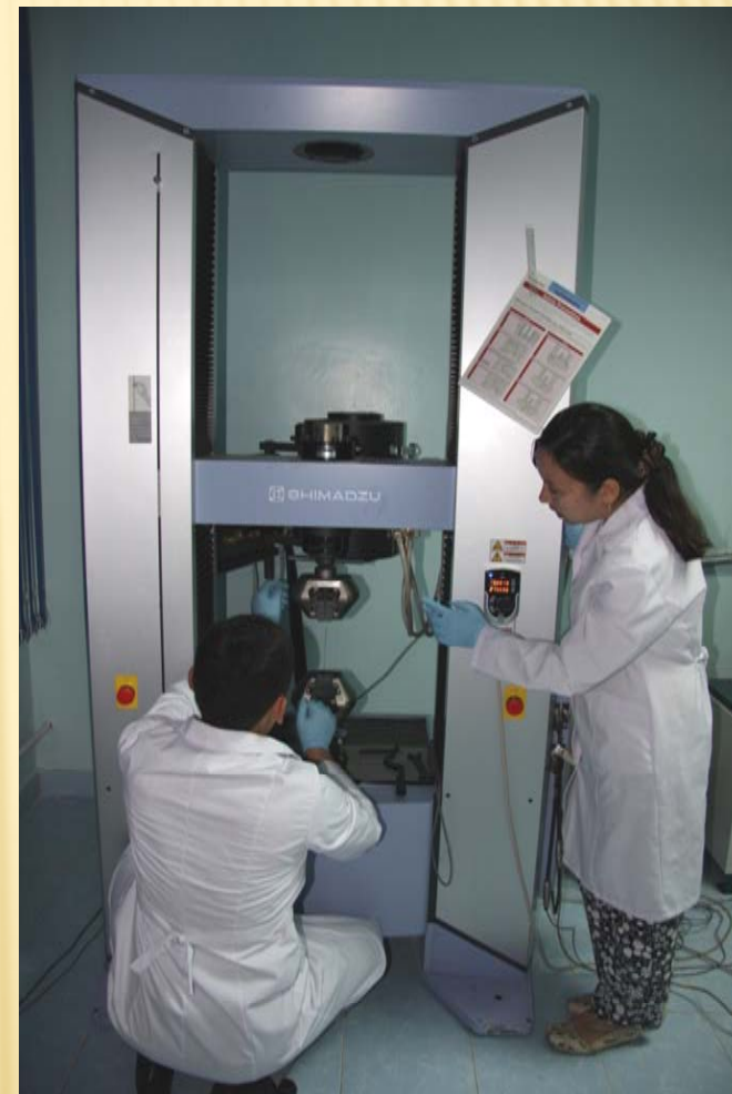
Universal electromechanical testing machine up to 100 kN Shimadzu AG-100kNx (Japan)
