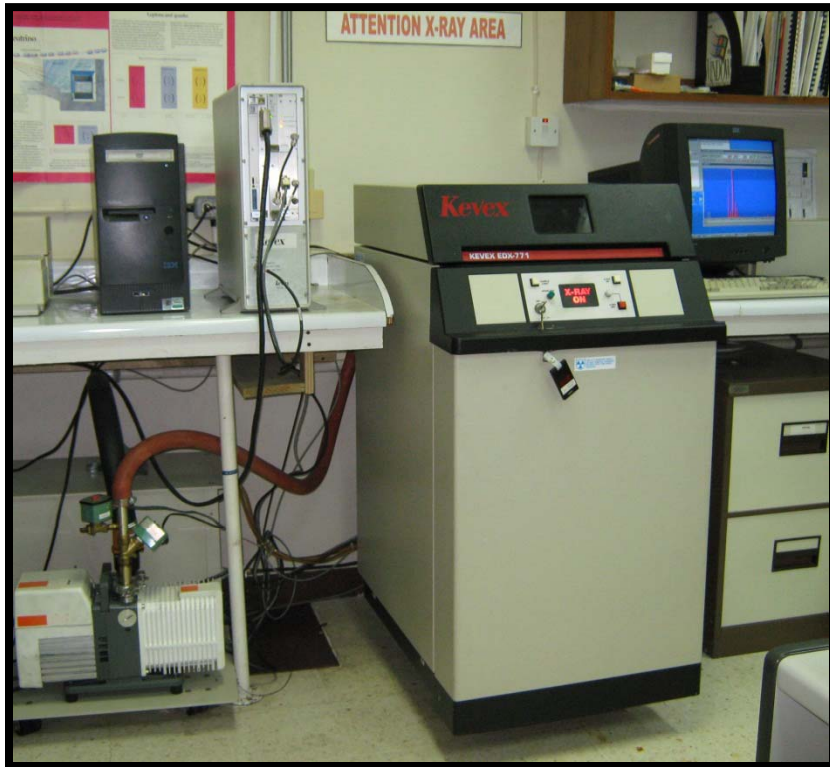
Kevex Spectrometer ED-771 XRF K, Ca, Ti, Cr, Mn, Fe, Ni, Cu, Zn, Rb, Sr, Y, Zr, Nb, Cd, Cs, Ba, La, Hg, Pb, Ce
