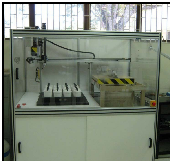
20% HPGe N detector with sample changer
