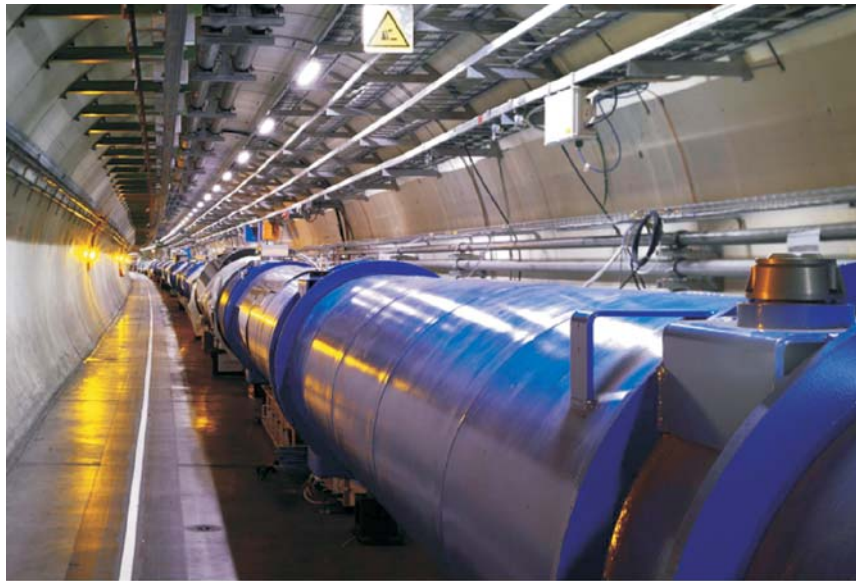
Figure - 1: The LHC tunnel between points 1 and 8, showing some of the large superconduction magnets (1232 dipoles with a field of 8.4 Tesla) that constitute part of the 27 km underground accelerator structure
